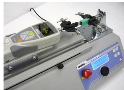
USB connector extraction / insertion (repetition) test
