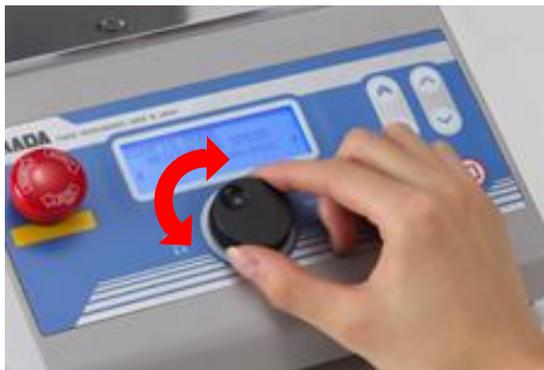
Adjusting moving distance with the limit nobs.
