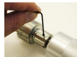
Turn screw by attached L wrench
