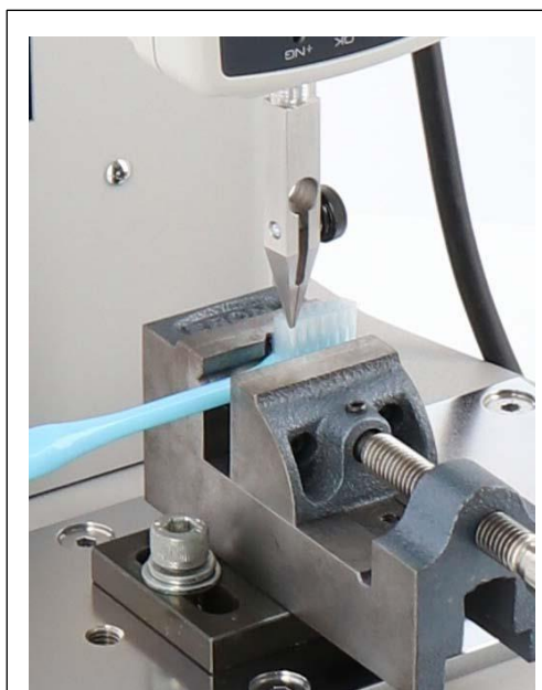
Test Image (Tensile strength test of brush)
